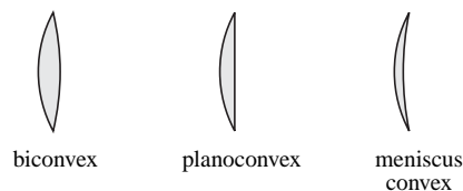
(a) Converging, positive, or convex lenses.
